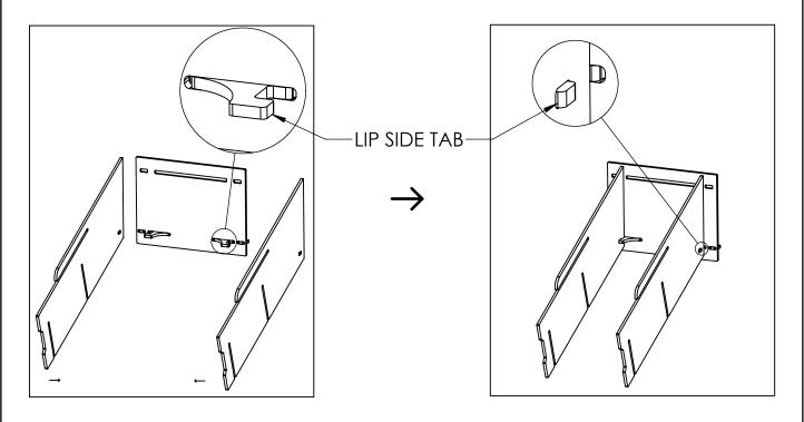
**STEP 3:** Slide the Back Panel into the long slots on the Side Panels until the tabs on the Back Panel engage the slots on the bottom of the Top Panel.
